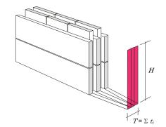
Where  $H \le 400 \text{ mm}$   $t_i.....$  Thickness of board layers in direction of mechanical actions  $\overline{t_i}$ ...... Thickness of board layers perpendicular to direction of mechanical actions V...... Shear force
